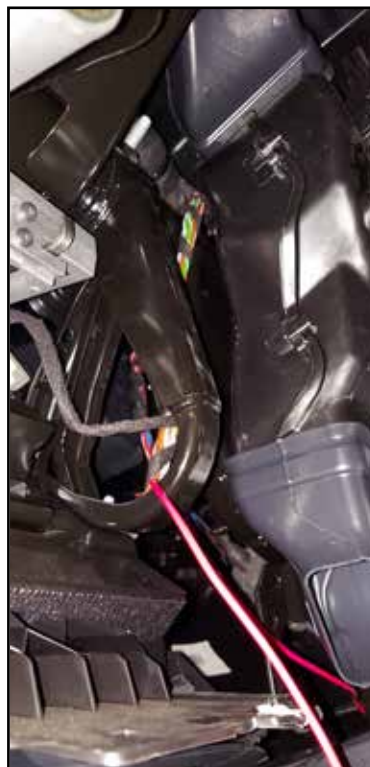
7) Route through steel loop and secure.
