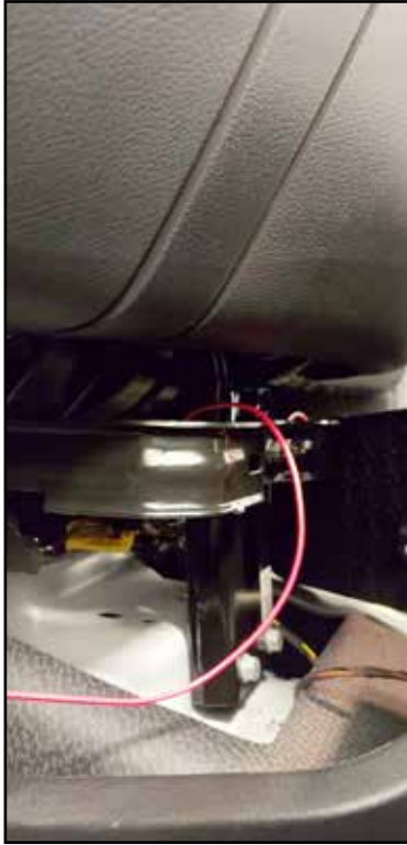
2) Routing after removal of shroud.
